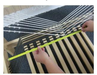
Check the position of the cords that connect the lams to the lower shaft bars. The location on the lams should be exactly in the middle. Replace the connection to the lams if necessary. Start with the ones in the front and the back, so the ones in between can be placed in line.
