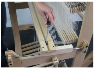
Remove the knurled nut from the threaded ends.
