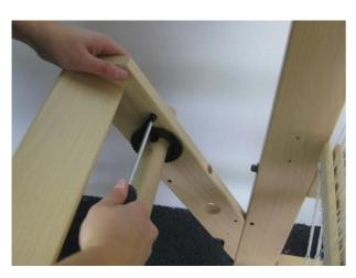
Install a ratchet next to the ratchet wheels of both beams. Use the round head screws 4.5 X 17 mm. Tighten them and then unscrew them just far enough that they can turn freely.
