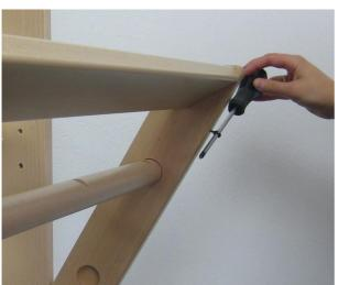
Screw the little screw eyes into the warp beam supports. Use a screw or something similar to twist it easily.
