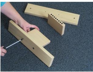
If your loom is a David 90, use the four 5x50 screws and attach the lam squares to the lower side rails at the same side where the holes for the barrel nuts are located.
