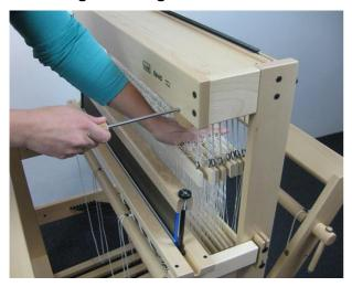
If you want to add heddles or to remove heddles from a shaft, you have to unhook cords from the shaft bars. This is easier after you have blocked the system by inserting the locking pen through the wooden discs. In this situation the springs give no tension on the system.
