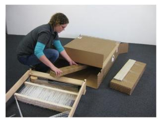
We have assembled the castle section of the David loom in the factory. Slide this assembly out of the box, after you removed the box containing all the parts listed on next page.
