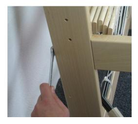
Put a threaded end through the hole in the upright. Slide the rail onto the threaded end and push its wooden dowels into the holes of the upright. Turn the threaded end into the barrel nut, while positioning the barrel nut, if necessary, using a coin or a screwdriver.
