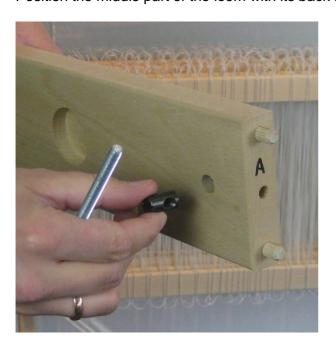
The uprights of the middle part are marked **A** and **B** at the location where they should be connected to the corresponding marked sides of the top side rails.
