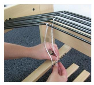
Hook the other end of the cord to the corresponding screw head of the treadle.
