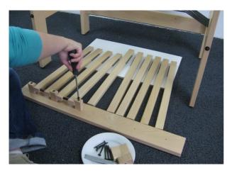
Assemble the treadles onto the foot rail. The screw heads on the treadles should point towards the middle so that the five treadles on the left side are opposite to the five treadles at the right side.
