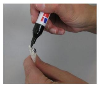
Use a felt pen to mark the center of the beam cords.
