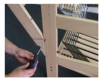
In both uprights at the back of the loom there is a hole in the location where the polyurethane dowels of the back part are inserted. With the two screws 3 X 20 (not the round head 4.5 X 17 ones) you will secure the polyurethane dowels.
