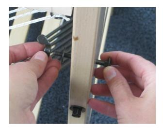
Insert a carriage bolt through the lower hole in the side of the main post, place the washer on the end and screw on the wing nut a few turns.
