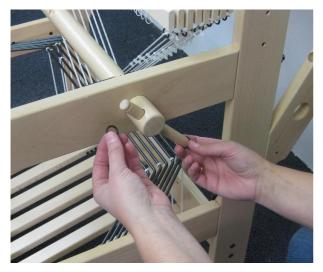
Insert the beam handles through the holes in the beams and secure them by rolling the rubber O-ring into the groove around the handles. A spare O-ring is in the hardware bag extra.
