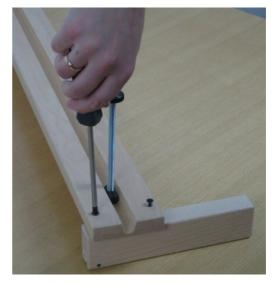
The picture at the left shows in what position the bearing blocks have to be connected to the reed holder. Note the direction of the slope of the notch. Assemble the blocks and the reed holder with the screws  $4 \times 40$  mm.
