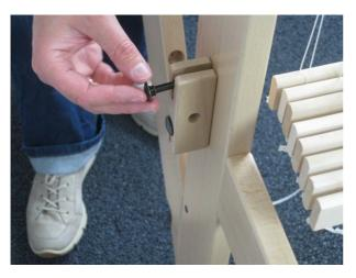
Slide the block with the two slots on the carriage bolt. Note that the oval hole faces the front of the loom. The second carriage bolt has to be plugged into the other slot and the other hole. After you've fastened the bolts with washers and wing nuts, mount the second block onto the post at the other side of the loom.
