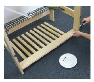
Put the foot rail with the treadles in between the front posts of the loom and connect these parts with the four remaining screws.
