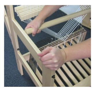
Install the cloth beam in the loom. First insert the side with the ratchet wheel into the hole in the side rail, while you keep the other end of the beam just above the opposite side rail. Because of the beam is slanted in this position, the hole is tight and you have to turn the beam while pushing it through.
